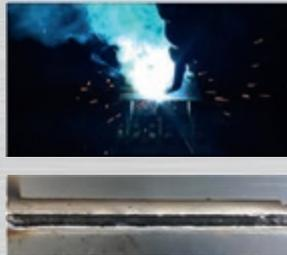
Improvement of the weld pool through widening the arc and using reciprocating wire feed and allowing a periodic and proactive de-gassing of the zinc layer.
